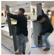
Strips are connected along edges to create a tube of any diameter. Each strip adds exactly 2 in. (51 mm) to the diameter of the tube. That is, 6 strips make a 12-in. (305 mm) tube, 7 strips make a 14-in. (356 mm) tube, etc.
